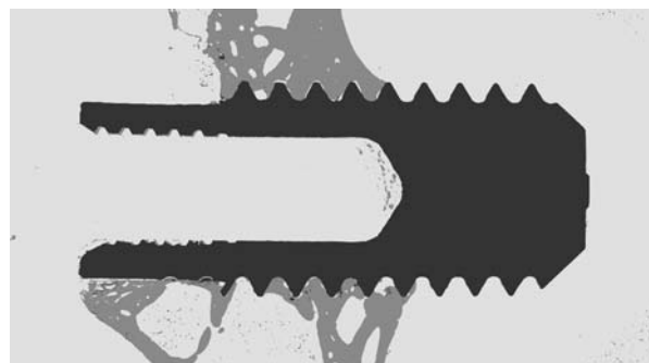
Fig. 4 Segmented image: the dark grey region corresponds to the implant, light grey areas to bone—all other pixels are white
